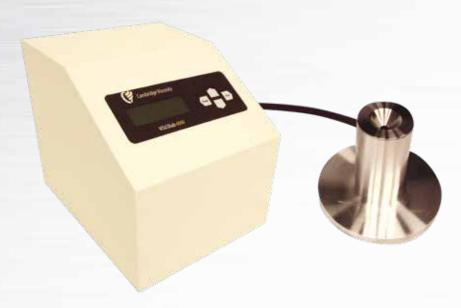
The Cambridge Viscosity ViscoLab 4000 Small Sample Viscometer utilizes oscillating piston technology and an embedded PT100 temperature sensor to provide exceptionally accurate viscosity and temperature readings.
